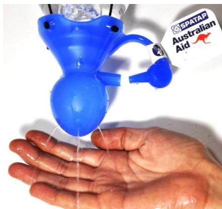
The SpaTap is a device that attaches to a plastic water bottle, allowing a bottle to be used as one-touch handwashing device. The SpaTap is affixed to an upside-down water bottle, which is suspended to provide gravity flow. The SpaTap is made from food grade, UV-stable silicone. The device provides 25 effective hand washes when fixed to a one litre bottle.
